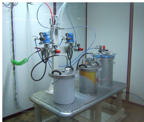
Water-borne paint supply, isolated of the ground potential, dedicated to electrostatic application with internal electrostatic charge.
