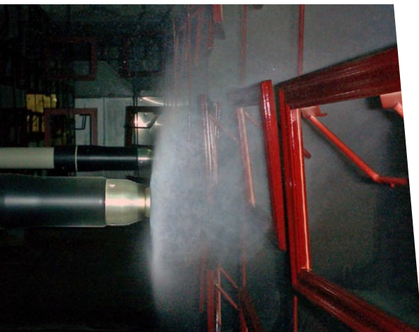
High speed bell, RPM 5,000 to 45,000 RPM, loaded
