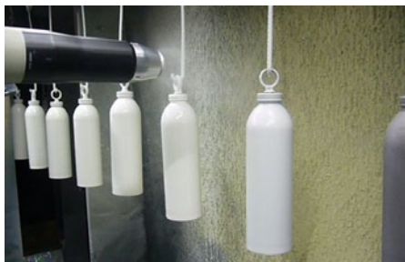
Water-borne paint supply, isolated of the ground potential, dedicated to electrostatic application with internal electrostatic charge.
