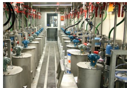
Water-borne paint supply, isolated of the ground potential, dedicated to electrostatic application with internal electrostatic charge.
