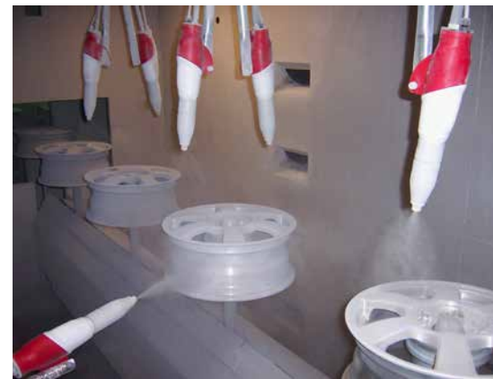
Application of a primer coat on aluminium wheels with Auto Mach-Jet sprayers
