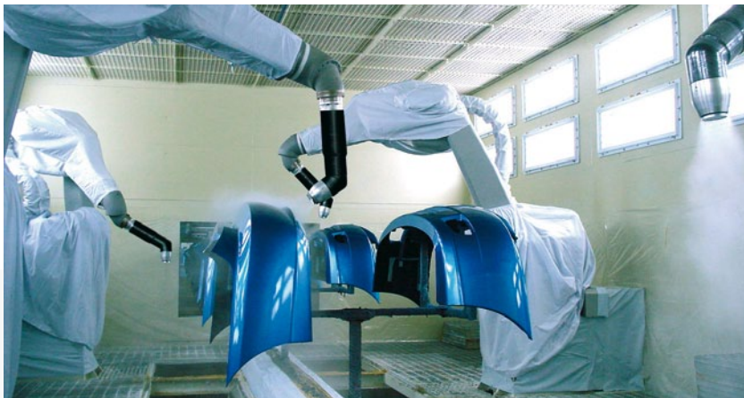
Clear coat application on bumper - PPH 707 SB
